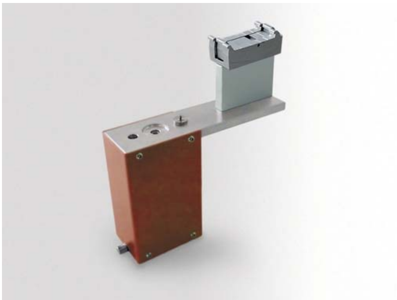
Figure 1. SPME Fiber Conditioning Station
